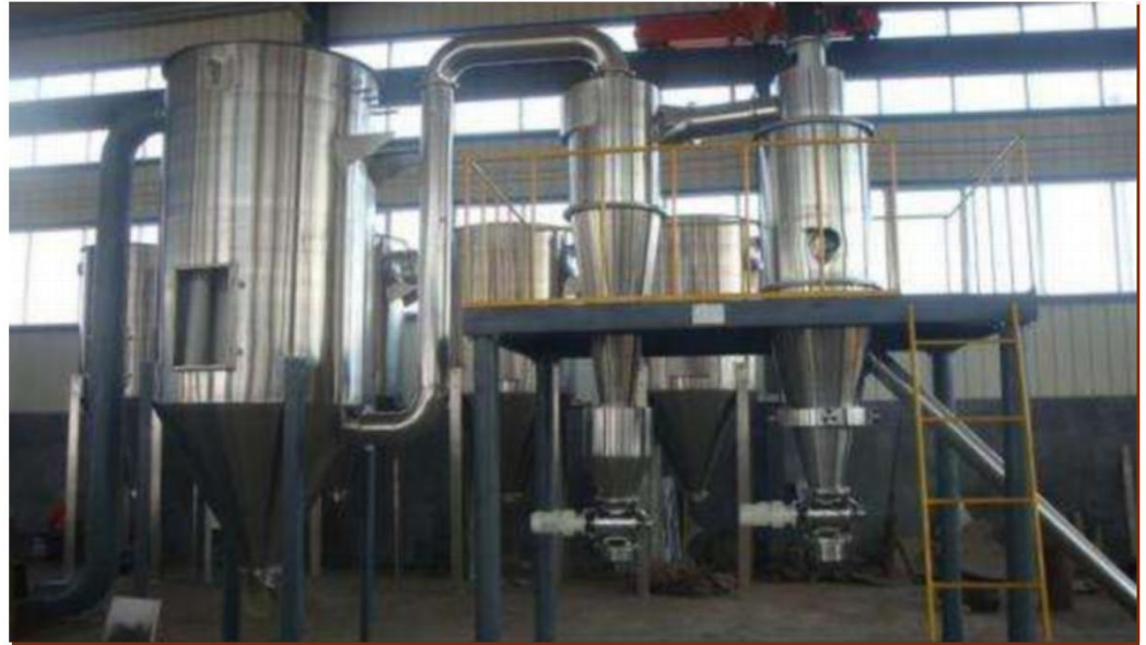
气流分级调整粉末粒度分布 Air grading adjusts the powder particle size distribution
