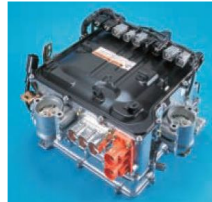
HEV Inverter Unit
